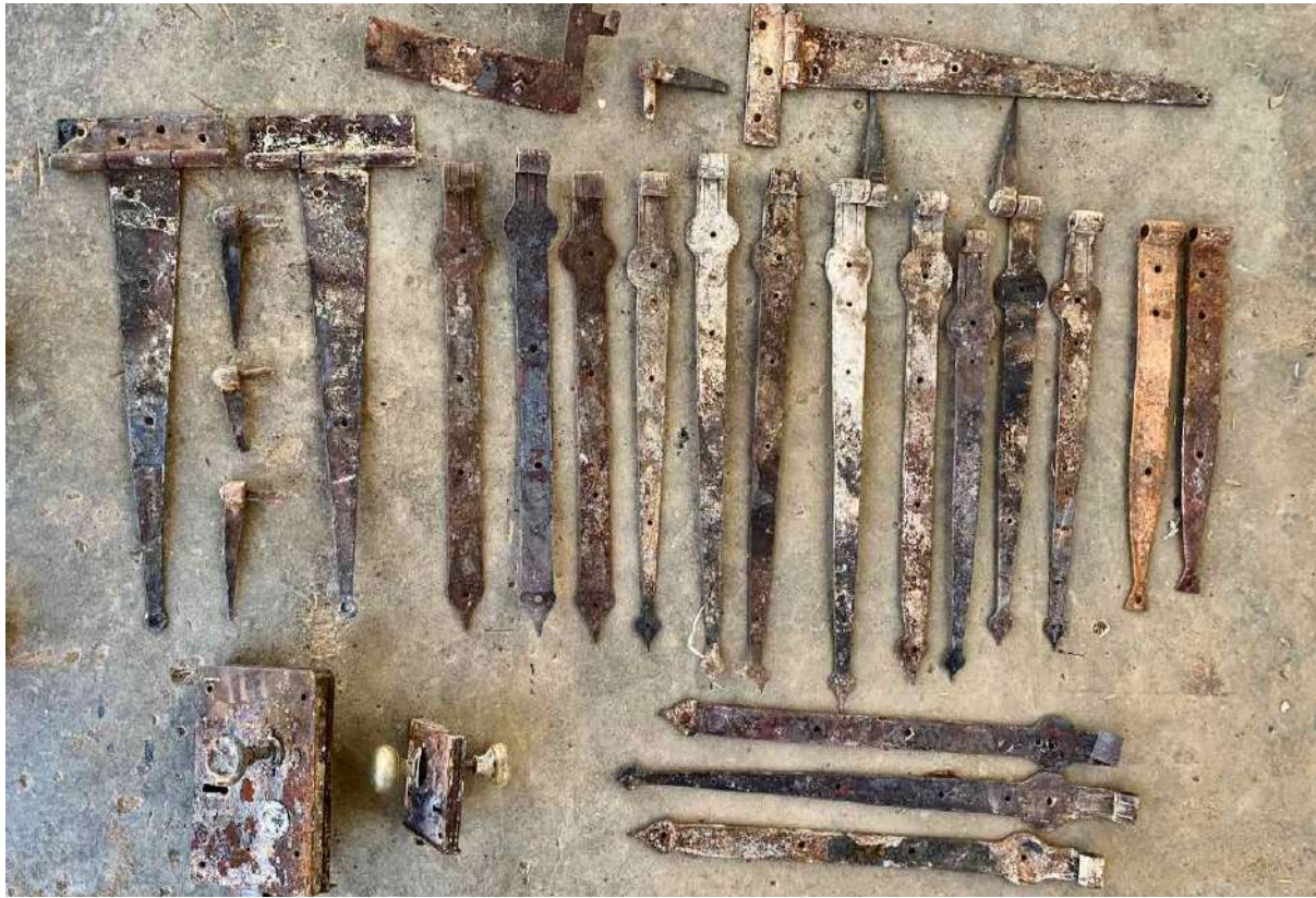
FIGURE 7: Examples of historic ironmongery recovered after the fire. These included a large 19 th C front door lock (bottom left). Most were recovered from the ashes and rubble of the Winkelhuis; and most, including the badly damaged and heat-seized door locks, were able to be reconditioned and reinstalled during the restoration project. (Image: ARCON, 24 January 2019).
