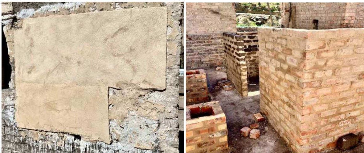
FIGURE 8: Trial panels using lime/sand mixes for plastering and laying brickwork. Left: Two separate lime plaster panels experimenting with water proportions. The shrinkage cracks in the lower panel show that too much water was added. Right: Trial samples of brick walls constructed using exclusively lime/sand mortars to convince an initially skeptical contractor that such lime mortars without Portland cement would be structurally sound. The wall in the foreground is constructed using modern fired bricks. The darker wall in the background experiments with bricks recovered from the fire damaged ruins. (Image: ARCON, 30 August 2019).
