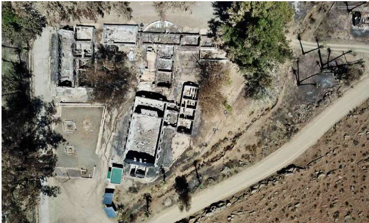
FIGURE 1: Aerial view showing the gutted state of some of the buildings in the town centre after the fire. Top centre are the remains of Leipoldt House with its T-shaped plan and semicircular stoep. To the left are the remains of the old Mission Stores building, the first school building in the settlement. Below are the remains of the Community Hall. The Old Blacksmith's Shop (Smitswinkel) where wagon wheels were repaired after a torturous trip down the mountain pass is just visible on the extreme upper right. The latter was the first building to be gutted in the fire. The road on the bottom right enters Wupperthal from the pass. (Drone image: Goal Zero Consulting).
