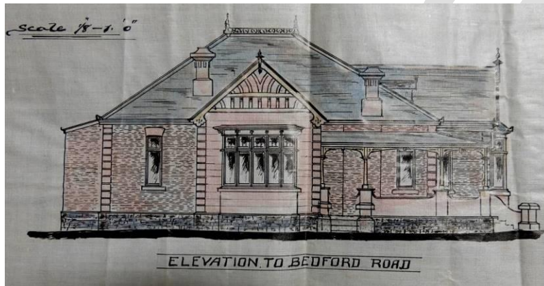
Fig. 56_Street elevation to Bedford Road with centrally located triangular decorative gable from 1906 (Source: Plans Department, City of Johannesburg)
